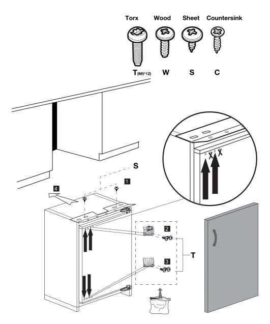
**Note:** Installation step for 2, screws for connecting the top plastic part should not be fully tightened until final left-right adjustment.
